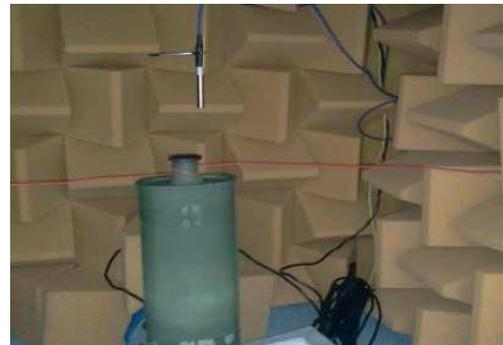
Fig. 3. Noise measurement of 'A' silencer
