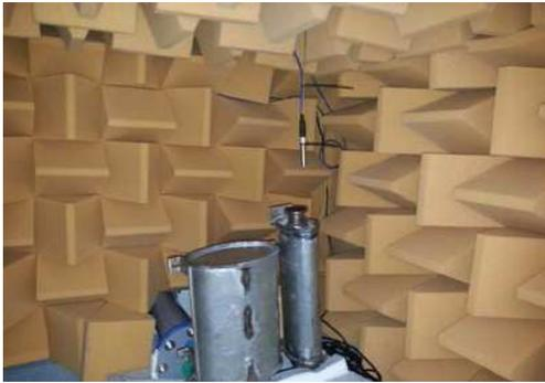
Fig. 4. Noise measurement of 'B' silencer
