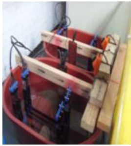
Fig. 6. Experimental set up of water absorption test
