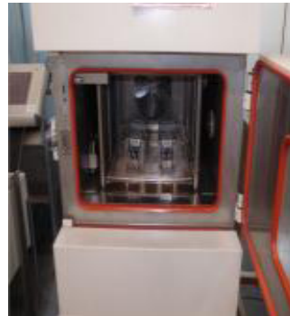
Fig. 10. Experimental set up of thermal cycling test
