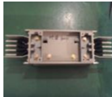
Fig. 11. Specimen for acceleration aging test
