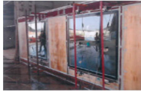
Fig. 5. Wind pressure test
