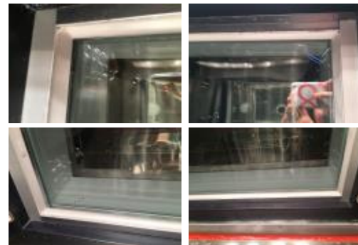
Fig. 14. Appearance of specimen after 400cycles (Silicone Sealant type)
