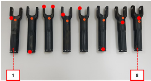
Fig. 6. Yoke tube samples with various cracks in them.
