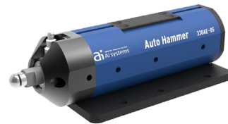
Fig. 5. Fabricated auto-hammer. Impact force could be varied. The cylindrical design made it to be compact and convenient. The size was 120mm × 38mm × 38mm.
