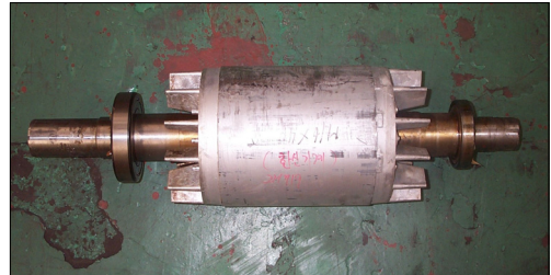
Fig. 1. Configuration of Induction Motor Rotor
