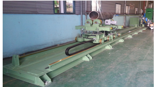
Fig. 12. Appearance of the developed PT inspection system
