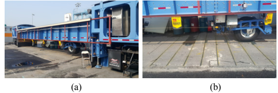
Fig. 9. Experimentation of wheel load (a) View of the APT (b) Application of wheel load
