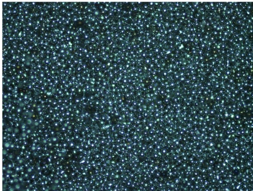
Fig. 3. Microscopic photo of stainless steel powder (AM 316L cl E) with the diameter size of more than 32 \mu\text{m}
