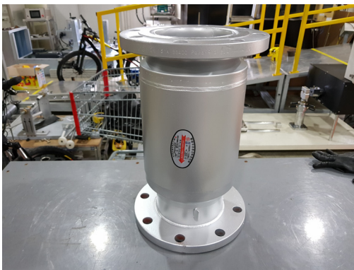
Fig. 1. Specimen : Bellows type expansion joint
