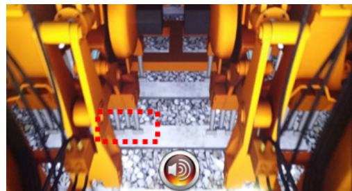
(b) Sleeper hitting due to human error
