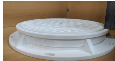
Fig. 13. Lifting state of manhole cover using 3D printed manhole assembly
