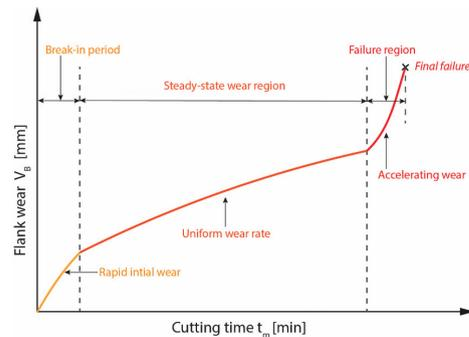
Fig. 1. Flank wear according to cutting time
