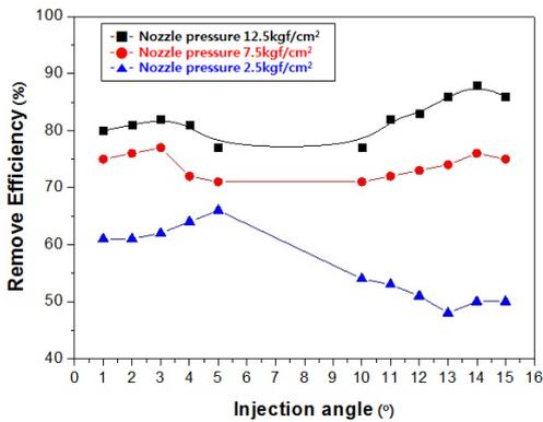
Fig. 9. Removal efficiency according to injection angle
