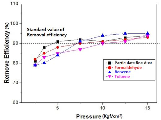
Fig. 8. Removal efficiency according to injection pressure by applying 2 mist nozzle
