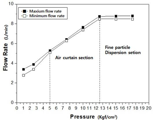
Fig. 5. Flow rate according to spray pressure
