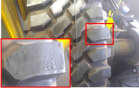
Fig. 4. Tire tread surface swelling caused by heat
