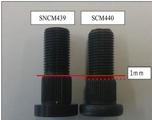
Fig. 5. Shapes of SNCM439 and SCM440 bolts
