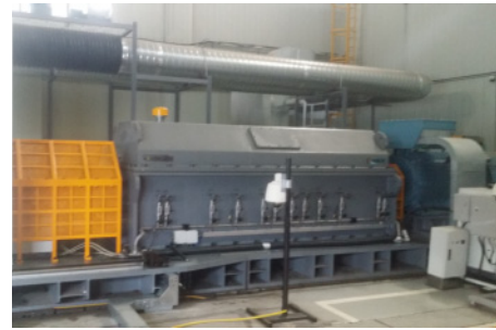
Fig. 3. Dynamo test bench
