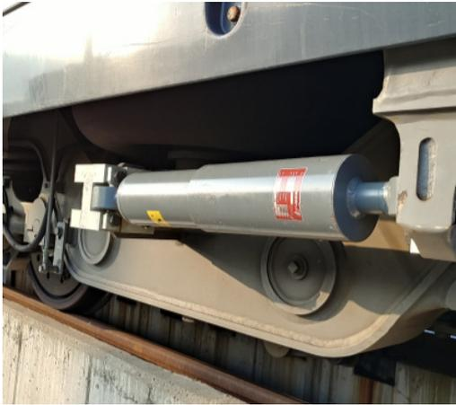
Fig. 7. Yaw damper angle adjustment
