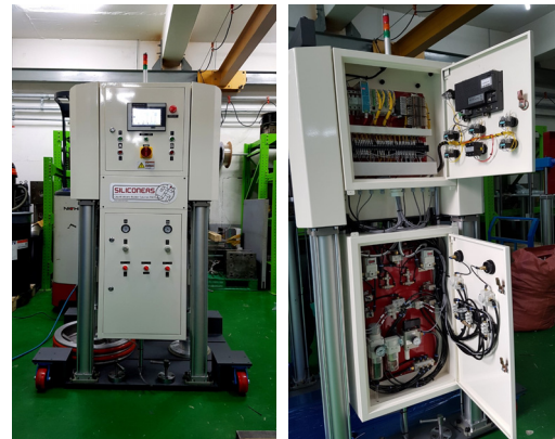
Fig. 7. Two-component liquid silicon mixing system
