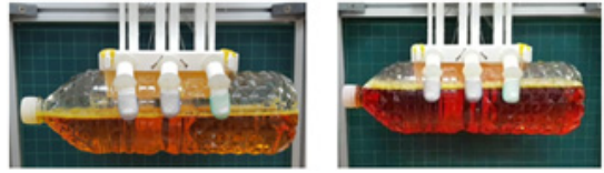
Fig. 11. Gripping test at 1000 g, and 1800 g
