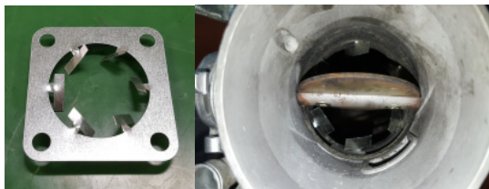
Fig. 3. Photos of manufactured gasket blade and mounted on intake manifold
