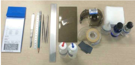
Fig. 9. Equipments for installation of strain gage
