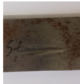
Fig. 4. Inflicted damage (Damage Case B-1).
