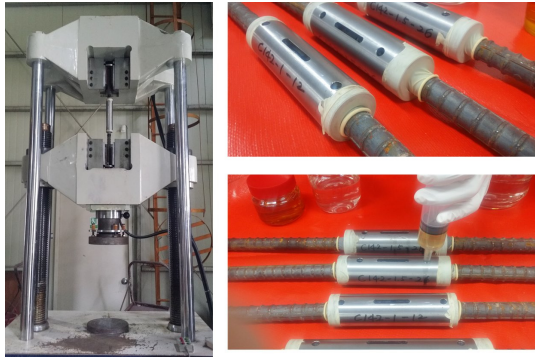
Fig. 6. UTM and Specimen of Mechanical Splice
