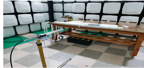
Fig 6. Radiated Emission Measurement setup
