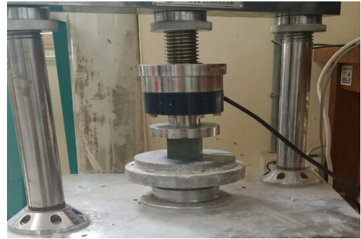
Fig. 4. Uniaxial compressive strength test
