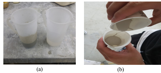
Fig. 1. Gel time test (a) A&B solution (b) Repetitive mixing
