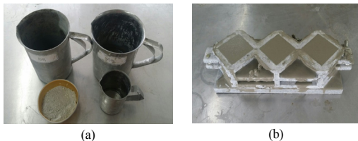
Fig. 2. Fabrication of test specimens (a) Specimen(A&B) (b) Grout curing
