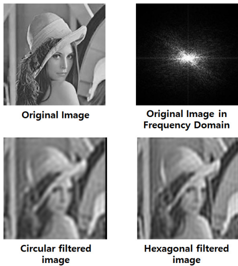
Fig. 6. Results of filtered image using circle and hexagon shaped filters
