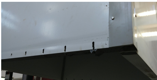
Fig. 10. Failure at bottom of "F" specimen
