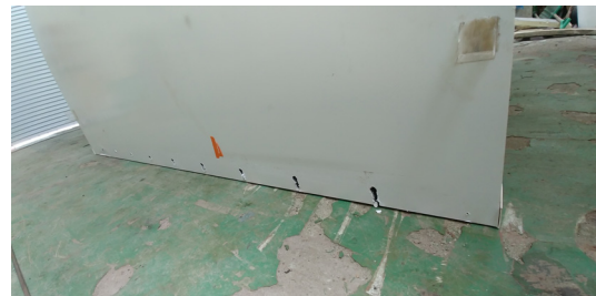
Fig. 12. Failure at bottom of cam lock specimen
