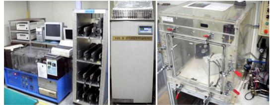
Fig. 8. AQS in gas measurement chamber
