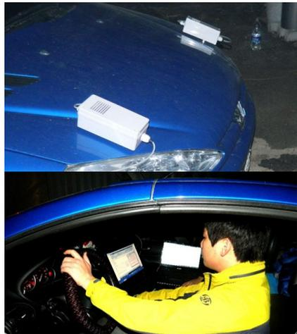
Fig. 13. Installation of AQS on the vehicle
