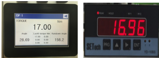
Fig. 6. Display of Target and measuring Torque
