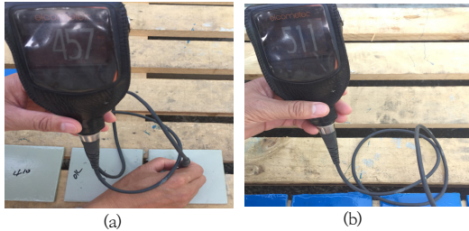
Fig. 3. Result on film thickness (a) EH 2350, (b) DuraTough DL
