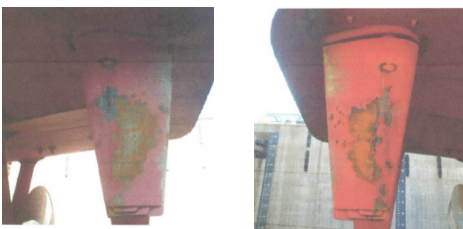
Fig. 1. The case of corrosion rudder of OO ship
