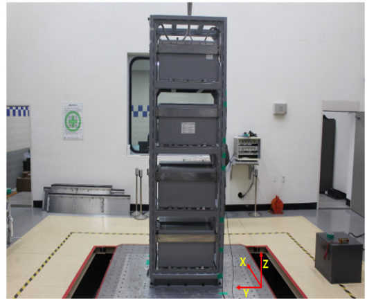
Fig. 6. Seismic Test Setting
