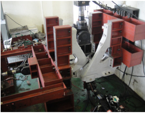
Fig. 8. Photo of the durability test for gangway ring
