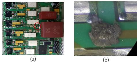
Fig. 3. IGBT Combustion
