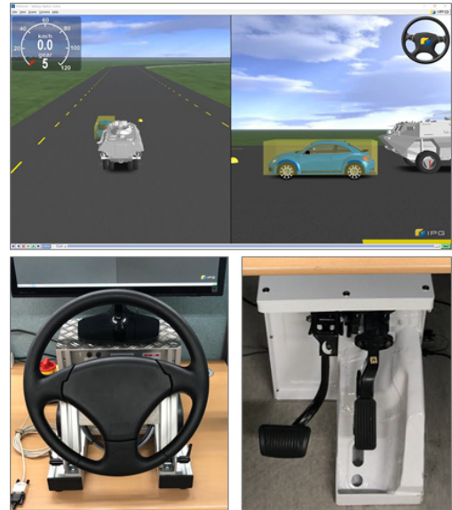
Fig. 11. Simulation: Forward Collision Situation
