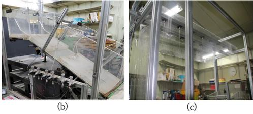
Fig. 1. Small-sized indoor landslide model equipment (a) Small-sized indoor landslide model pattern diagram (b) Small-sized indoor landslide model (c) Artificial rainfall system
