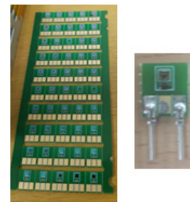
Fig. 6. Fabrication Process of the capacitive humidity sensor
