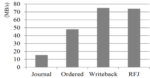
Fig. 8. Throughput comparison to the default journaling modes in the Ext3 File system. Result of File server workload in the Filebench.
