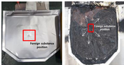
Fig. 7. Battery cell foreign matter Short Circuit test
