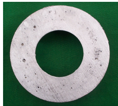
Fig. 11. Sectional view of lower end ring cast
