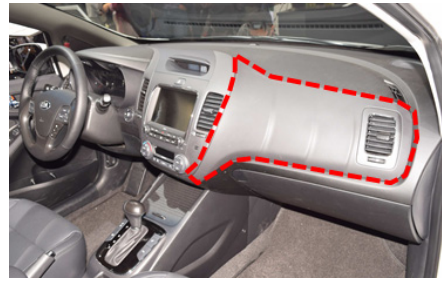
Fig. 1. Applied part of IMG integral foaming crashpad
