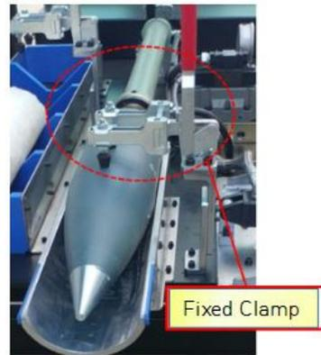
Fig. 8. Ammunition clamping
