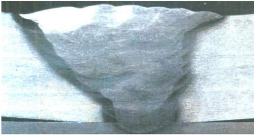
Fig. 11. Welded part macro test result(2G)
