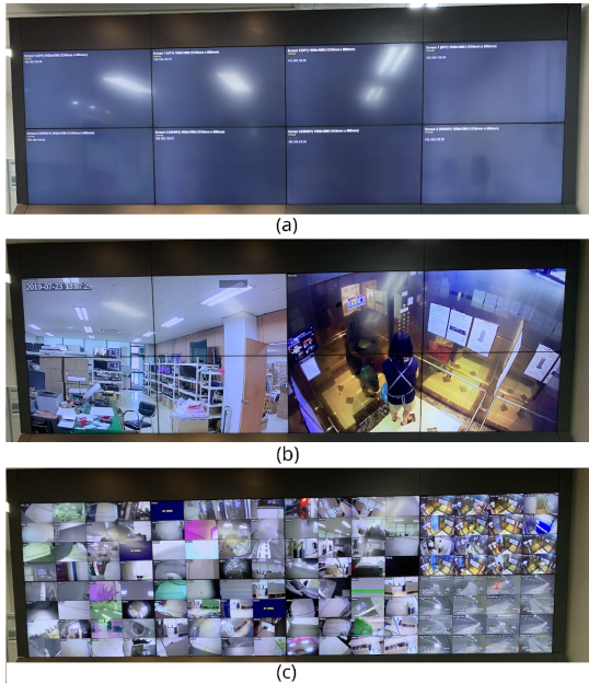
Fig. 6. IP Video Wall in Action (a) Initial 4x2 monitor screens (b) 2 videos in 2x2 scaling mode (c) 16x8 videos in 8 monitor screens
