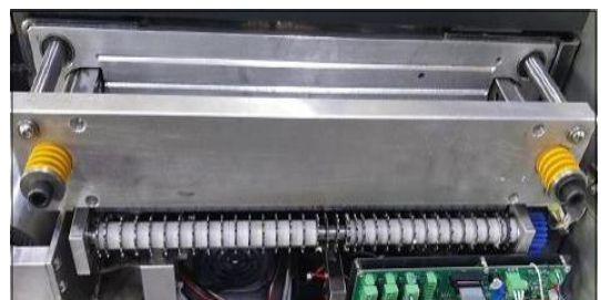
Fig. 4. Scarfing roller part of adhesive wireless bookbinding machine
