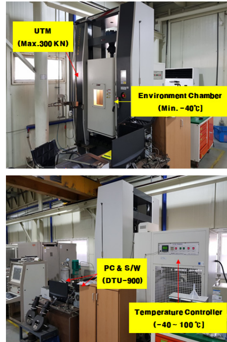
Fig. 3. Test equipment for low temperature tensile test
