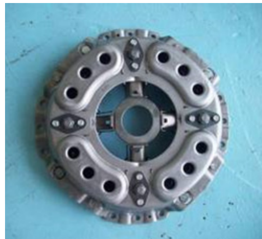
Fig. 7. Improved clutch cover including center ring
