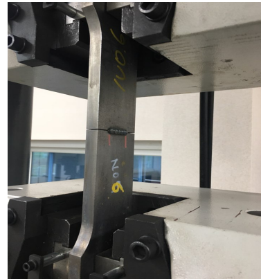
Fig. 7. Tensile test of deep-notched test specimen repaired by screws
