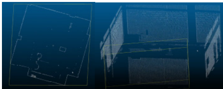
Fig. 4. Geometry segmentation from 3D point cloud
