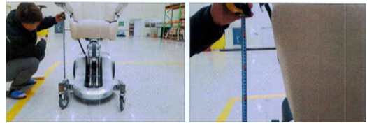
Fig. 23. Maximum lifting height measurement experiment
