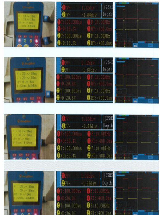
Fig. 27. Duty cycle error rate of control part and drive part
