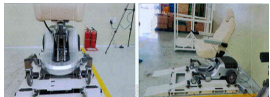
Fig. 20. Jig used to measure continuous travel time
