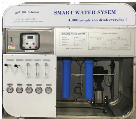
Fig. 3. Implemented groundwater purification apparatus
