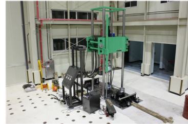
Fig. 6. 1000kN Dynamic material testing machine
