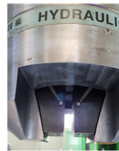
Fig. 7. Hydraulic grip jig for pullout tests
